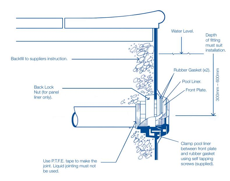
**Important:** All pipework and pool fittings must be pressure tested before backfilling and commissioning. Drawing is not to scale.
