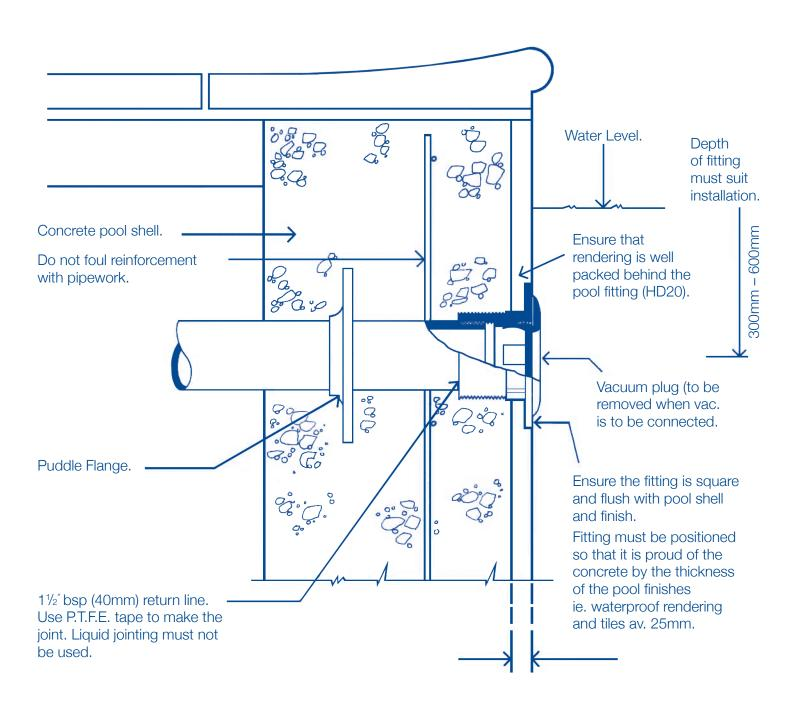
**Important:** All pipework and pool fittings must be pressure tested before backfilling and commissioning. Drawing is not to scale.
